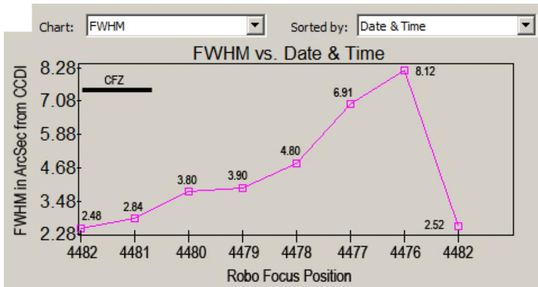
**Figure 4. Average FWHM analysis of images shown in Fig. 1 using the green filter.**
